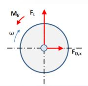
$$C_D, C_L, C_{Mz} = f(\text{Re}, X)$$
